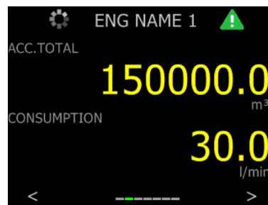
Figure 50: Menu 2 with Alarm warning
