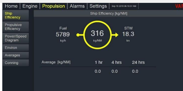
Figure 37 – Propulsion Ship Efficiency screen
