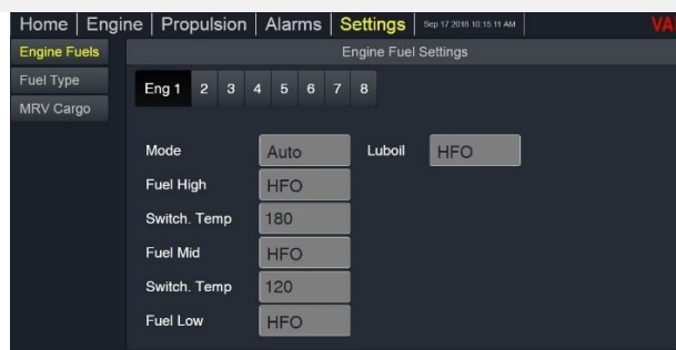
Figure 56 – Fuel type screen: Automatic fuel selection
