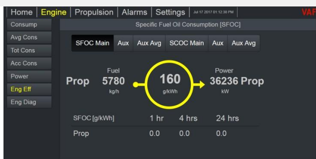
Figure 32 – Engine Efficiency screen single screw
