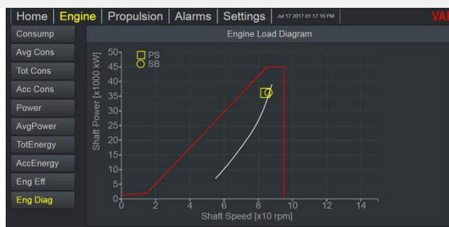
Figure 36 – Engine Diagram screen twin screw
