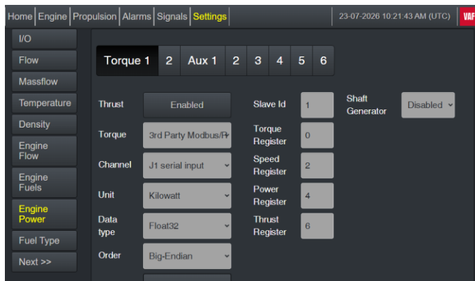
Figure 62 Setting up one or two 3 rd Party torque meters
